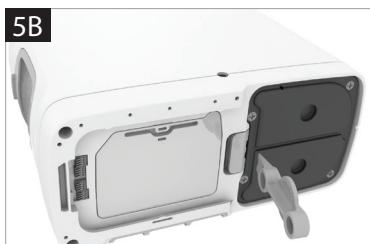
6. A. While holding the button open, slide the column assembly out of the device by pulling on the column pull handle or
