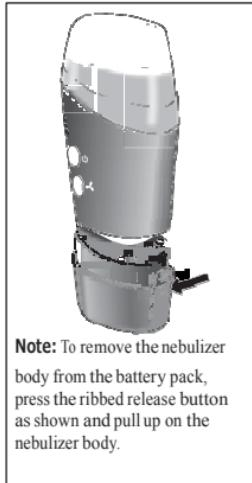
**Note:** To remove the nebulizer body from the battery pack, press the ribbed release button as shown and pull up on the nebulizer body.
