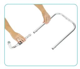
3. Slide the inner openings on the Crossbar © over the upturned ends of the two Elbow Rails (B) so it is sitting on the spring locking pins. Push one set of pins in and move that side of the crossbar down to cover them. Repeat on the other side, pushing the entire Crossbar down until the pins on both sides pop into place.
