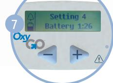
Set the flow setting to the flow rate prescribed by your clinical professional. The flow setting can be changed by pressing the triangular flow setting buttons that are marked with "+" and "-" symbols. Position the nasal cannula on your face and breathe normally through your nose.
