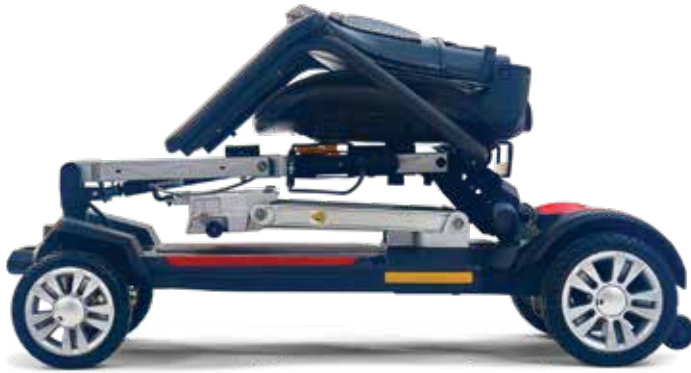
Tiller & self-locking seat frame fold for a compact profile
